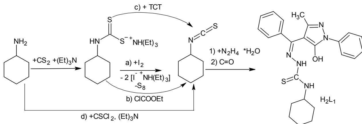
**Figure no. 1. Scheme of synthesis  $\text{H}_2\text{L}_1$ .**
