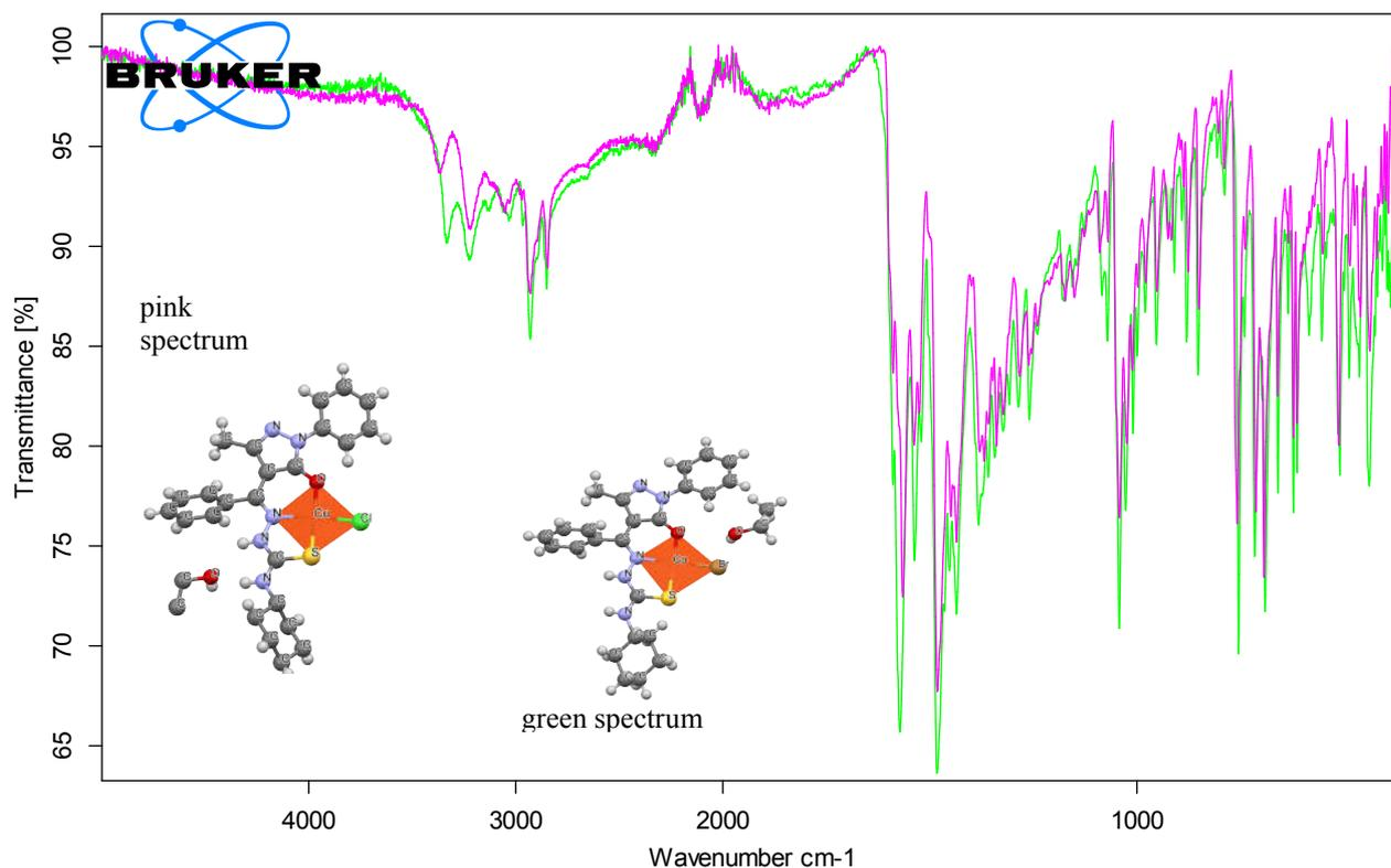
Figure no. 8. FT-IR spectra of compound  $[\text{Cu}(\text{HL}_1)\text{Br}]\text{C}_2\text{H}_5\text{OH}$  -green spectrum, and  $[\text{Cu}(\text{HL}_1)\text{Cl}]\text{C}_2\text{H}_5\text{OH}$  - pink spectrum
