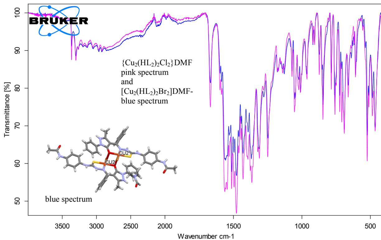
Figure no. 7. FT-IR spectra of compound  $\{\text{Cu}_2(\text{HL}_2)_2\text{Cl}_2\}\text{DMF}$ -pink spectrum, and  $[\text{Cu}_2(\text{HL}_2)_2\text{Br}_2]\text{DMF}$ - blue spectrum
